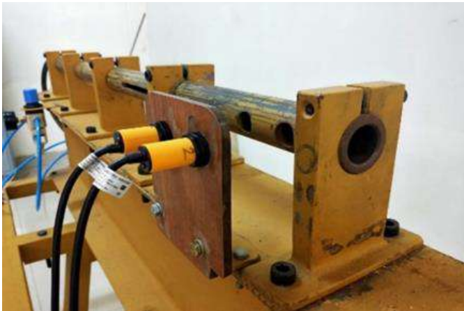
Fig.3.1 IR sensors mounted near the gun barrel
