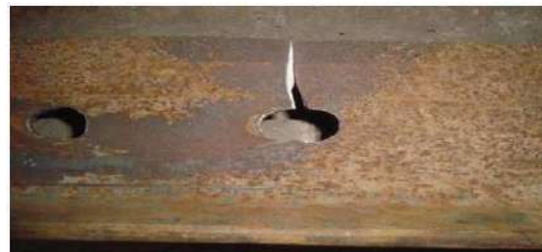
Fig. 4.1 Partial net section ruptures, with small eccentricity
