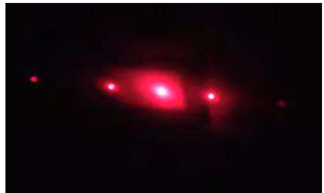
Figure 6. Order of LASER beam spots when diffraction taking place from plane diffraction grating.
