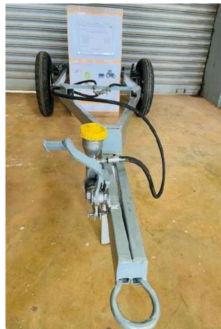
Fig 7: Trailer Disc Braking System
