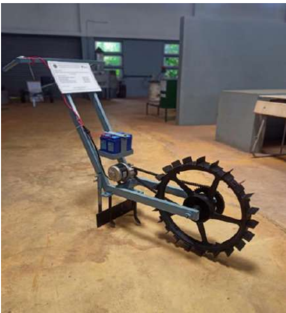
Figure 1. Portable Electric Ploughing & Levelling Machine
