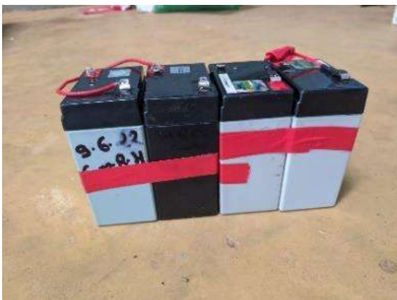
Fig 3.3: Rechargeable lead acid battery
