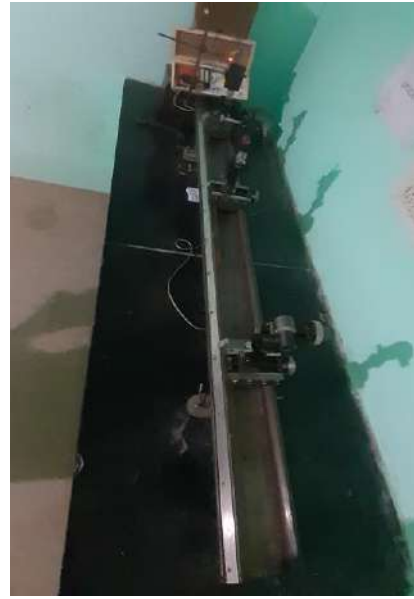
Figure 1: Experimental setup Solar energy dependent determination of wavelength using LASER source with optical bench.
