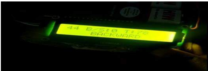
Figure 7-4 Display showing BACKWARD movement
