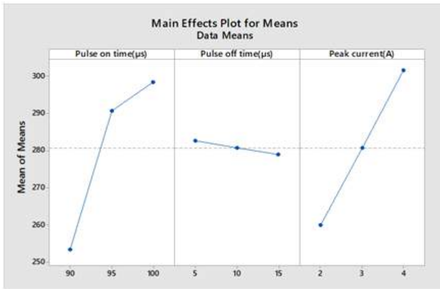
Fig.4: Main effect plot for kerf width
