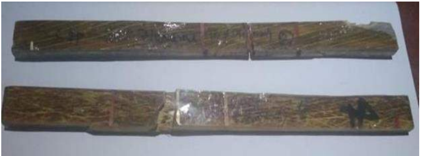
Fig.15 Flexural specimen after testing
