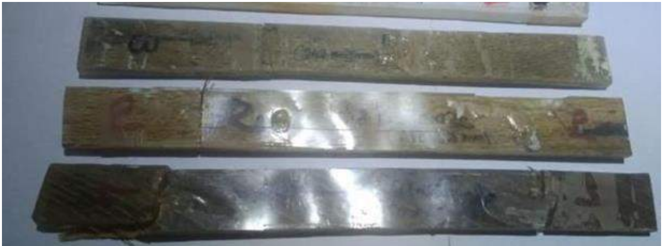
Fig.14 Tensile specimen after testing
