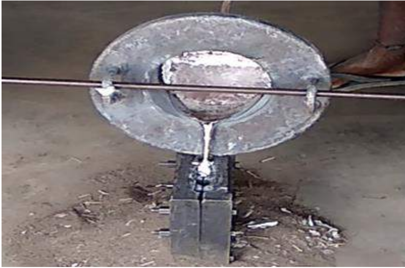
Figure 1: The specimen with varied reinforcement composition before being poured into molds
