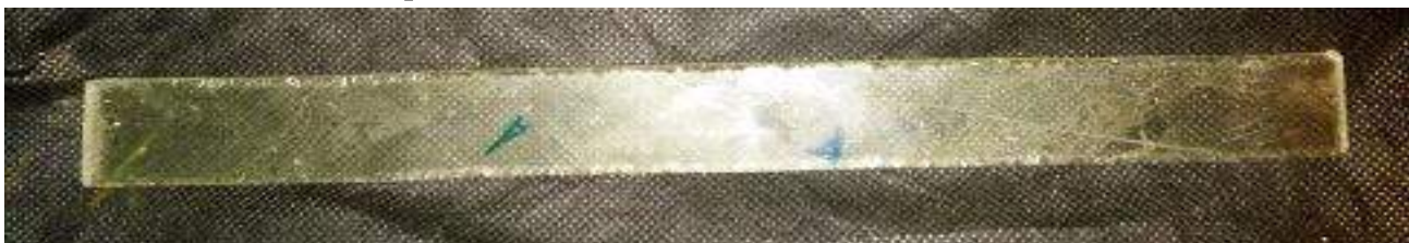
Fig.9 Tensile test specimen 100% epoxy resin Tensile specimen 250mmX25mmX5mm
