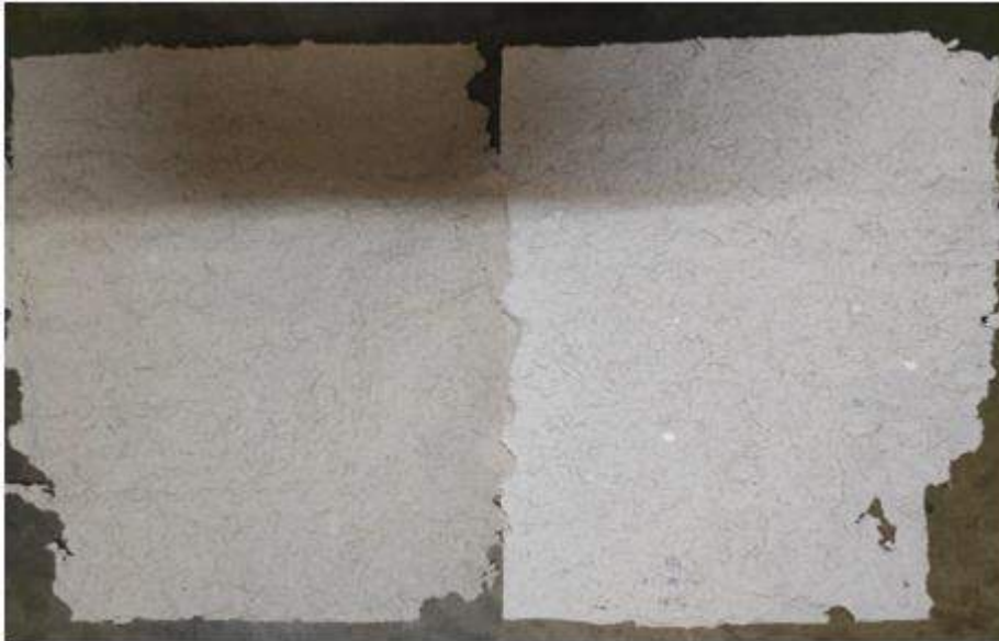
Fig 6: Sample paper of 80% coir: 20% Paper (Left) and 20%coir : 80% paper (right)
