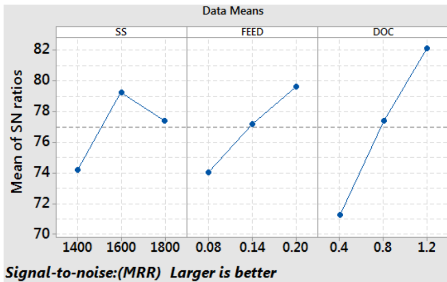
Figure 4: Main effect of SNR versus control factors
