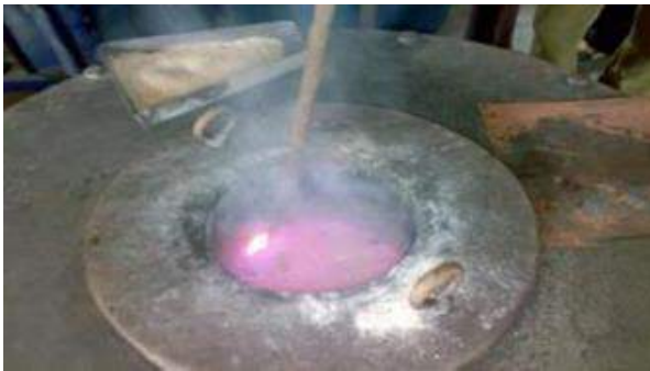
Fig.5 Degasifier is mixed in crucible
