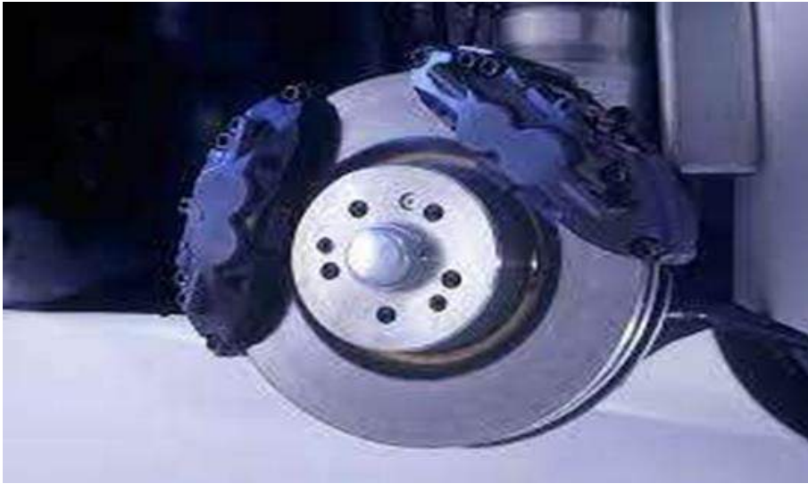
Disc Brake coupled with dual calipers[13]
