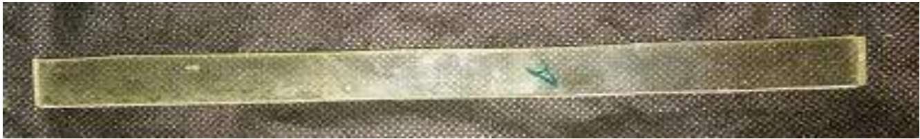
Fig.10 Flexural test specimen 100% epoxy resin Flexural specimen 200mmX15mmX5mm
