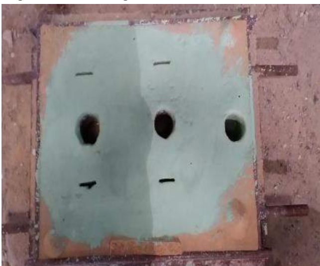
Figure 4: Mold box ready for pouring
