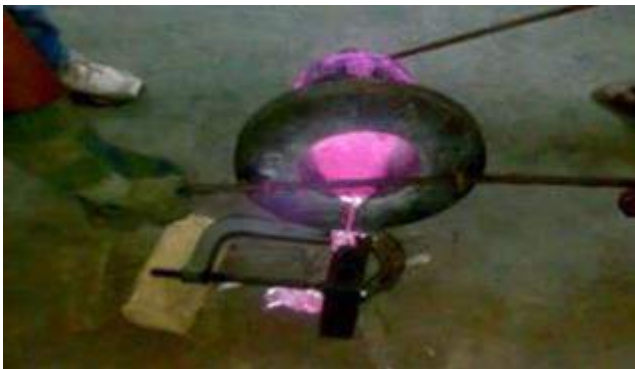
Fig.10 Hot liquid molten metal is pouring.
