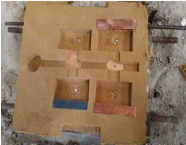
Figure 2: (a) Mold cavities with different end chills
