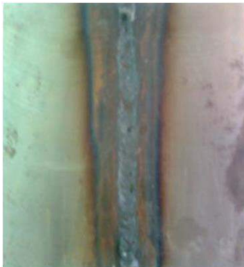
Figure.6:porosity and underfill.
