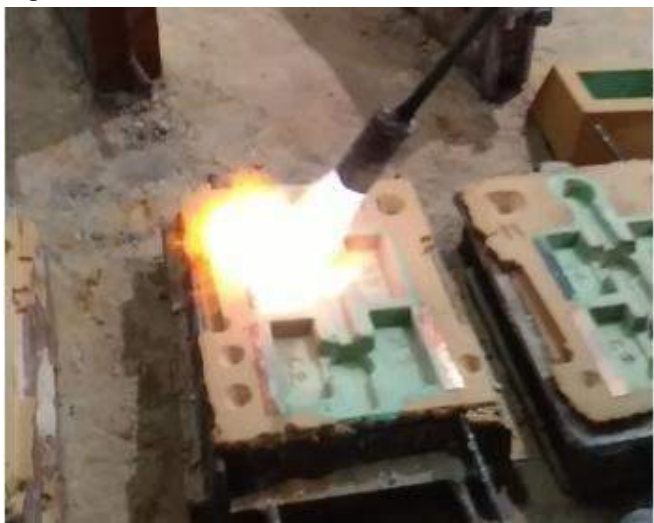
Figure 3: Preheating the Molds
