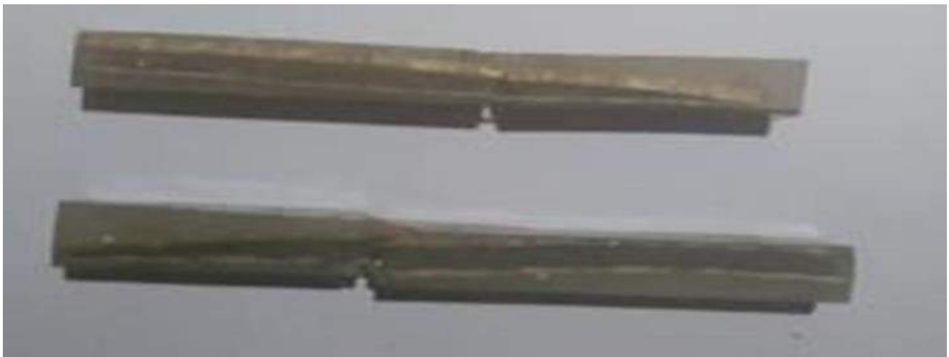
Fig.16 Impact specimens after testing
